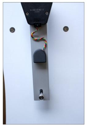
• Remove the encoder and fix the anchor bolt's foot with screws provided:
