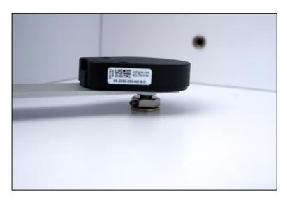
• Insert the anchor bolt into the slot on the encoder's arm, mark its place with a pencil:
