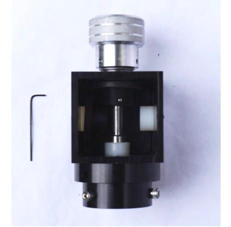
Now tighten the set screws on the encoder disk using 1.5mm Allen key (5) – just lightly (the encoder disks have a very tight fit). You may need to loosen the adjustment knob to be able to rotate the shaft to gain access to other set screws.
