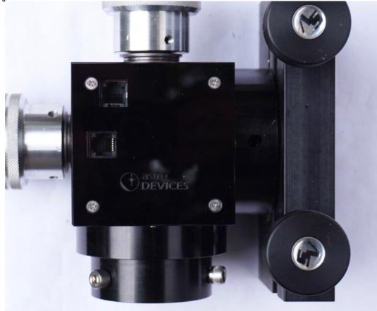
You will need the 2mm Allen Key (4) now. Press the bottom of the plate and tighten the set screw at the bottom first:
