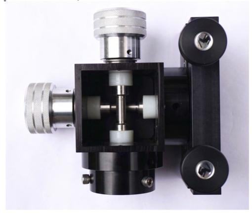
Now unscrew the tension adjustment knobs from both shafts and remove the thrust bearings and washers, then remove both shafts from the mount:
