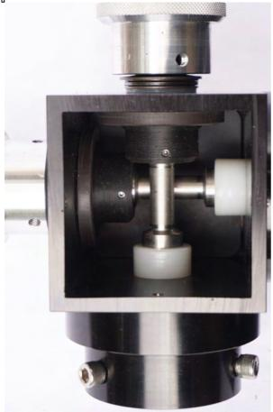
Now insert the encoder sensors plate – you should not need any force. The plate should only be inserted in the orientation shown below:
