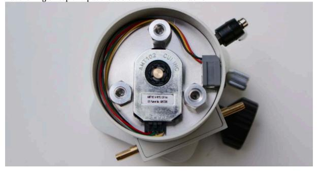
Place the assembled altitude encoder under the mount arm, put the screws back in and tighten them:
