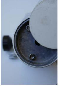
Remove the screws using the allen key supplied with the mount:
