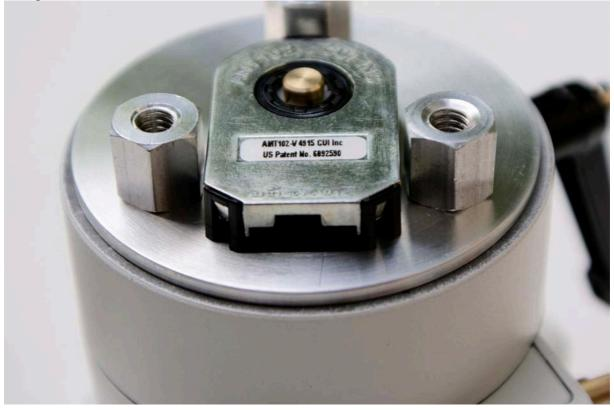
Plug the connector into the encoder:
