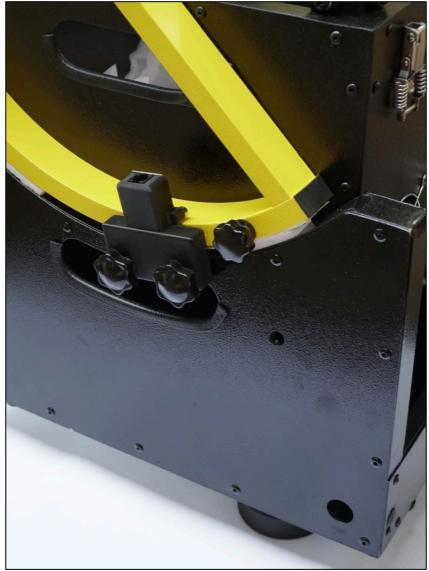
Position the telescope vertically. Now you need to use a pencil to mark the start of the magnetic tape – it should be approximately 10-15mm ( $\sim 1/2''$ ) from the right side of the reader:
