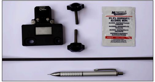
Put the mirror box into the rocker box and clean the internal surface of the altitude bearing (on the same side as where the focuser is) with the alcohol wipe:
