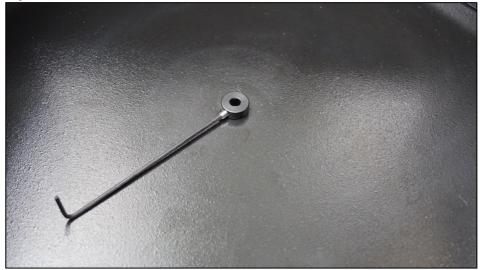
Clean the surface in the back with an alcohol wipe – where the encoder's foot will be glued. Remove the protective film from the encoder's foot:
